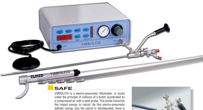
Since only compressed air pulses is the source of the impact effect, no heat is exposed. Therefore, there is neither risk of any thermal injury on tissue nor destruction on optics of endoscopy.
