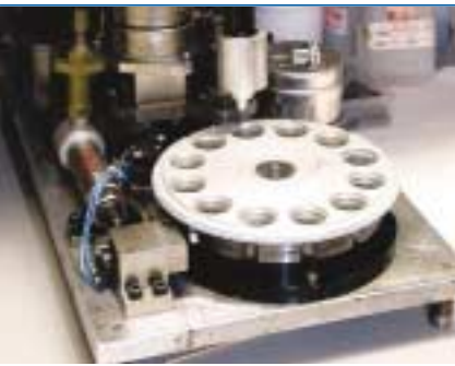
Lenses secured by highly precise automated adhesive dispensers
